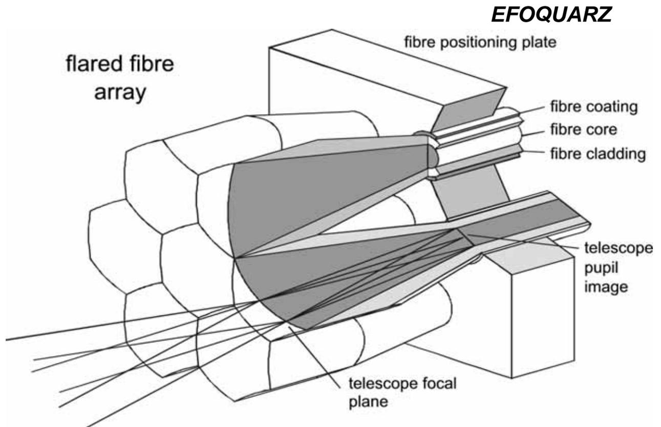
Picture 6: 3-D view of a tapered fiber-lens bundel
