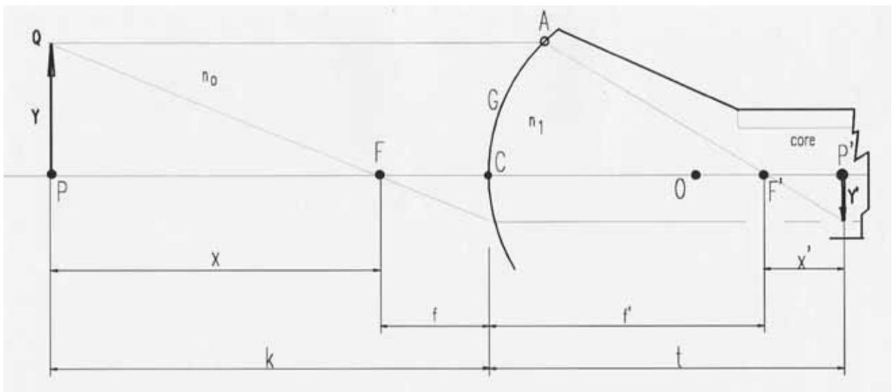
Picture 4: The object PQ is reproduced through the collimator lens onto the focal plane P Q. Expander used for Adaption
