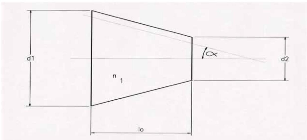
Picture 5: The correlation of the exit cross-section to the entry cross-section determines the beam expansion.
