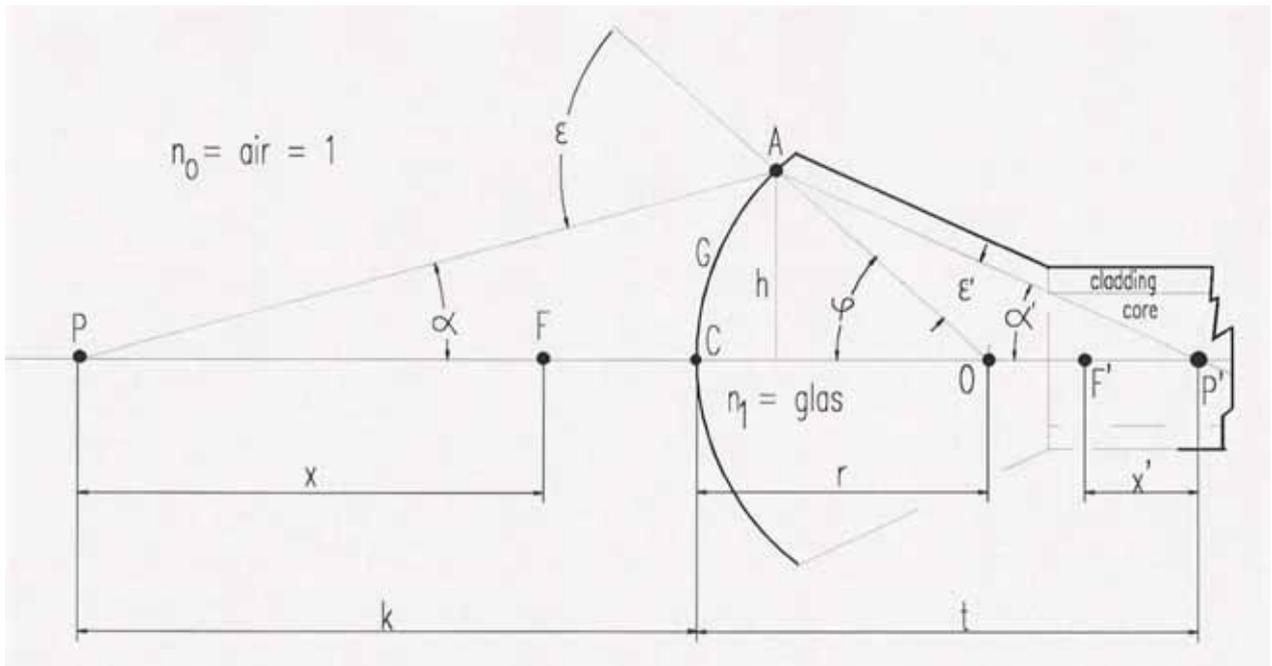
Picture 3: Beam refraction at the bended surface of the collimator lens.
