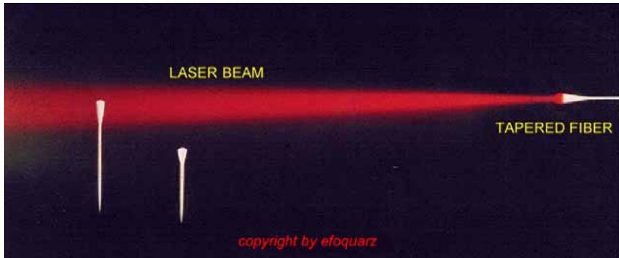
Picture 1: Focused laser beam and taper with integrated micro lens. The distance between taper and the exit point of the laser beam is 100 mm
