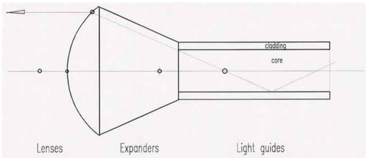
Picture 2: Lens taper consisting of a micro lens, a conical expander and the lightguide. All three optically effective components are made of pure quartz glass.
